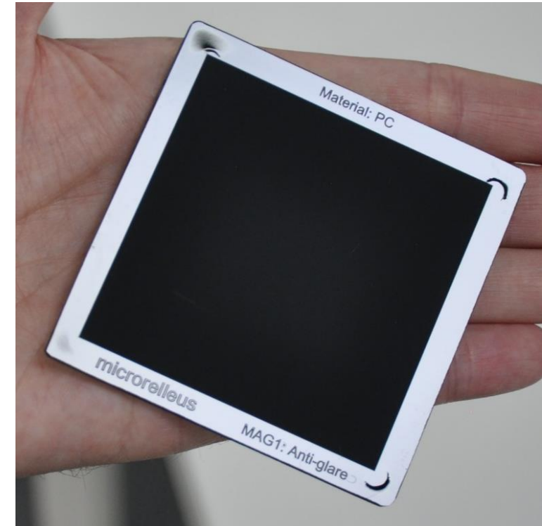
Anti-glare parts by engraving the tool
