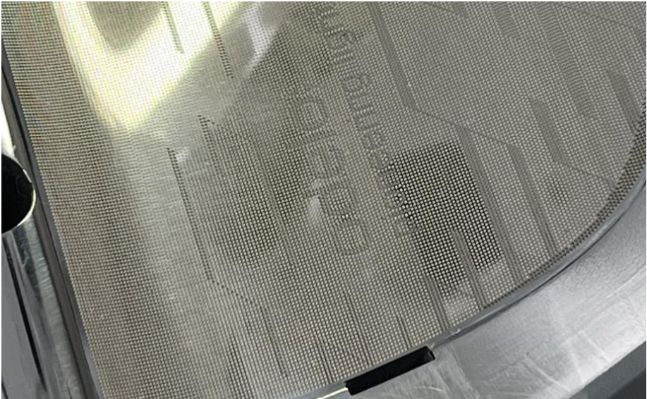
Engraving of thousands of microprisms in the production tool insert – free-form geometry
